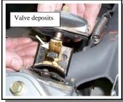
moderate restriction due to deposit formation can render the valve in-operable. In order to maintain peak performance, periodic maintenance is required. Within the snow-mobile industry, some recommend that valve maintenance (cleaning) be performed as frequently as after every 500-1,000 miles of operation.
