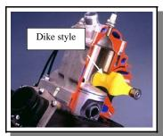
to activate the valve while others use an electro/mechanical method. A third style uses a direct cable or mechanical linkage to operate the valve. Though each design has its own benefits and disadvantages, all suffer from a similar problem. That problem, is that they all require periodic maintenance.
