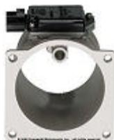
As air flows past the sensor element, it cools the wire and increases the current needed to keep the element at its operating temperature.
